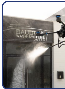
Baudoin Wash Drone Max. allowed take-off weight: 15,8 kg
