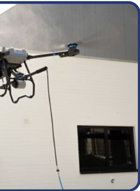
Wash Drone 2.6 Take-off weight: 58 kg
