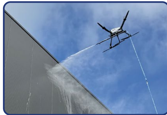
Baudoin Wash Drone 1.65 Max. allowed take-off weight: 15,8 kg
