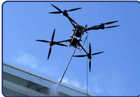
Baudoin Wash Drone 3.0 Max. allowed take-off weight: 95 kg
